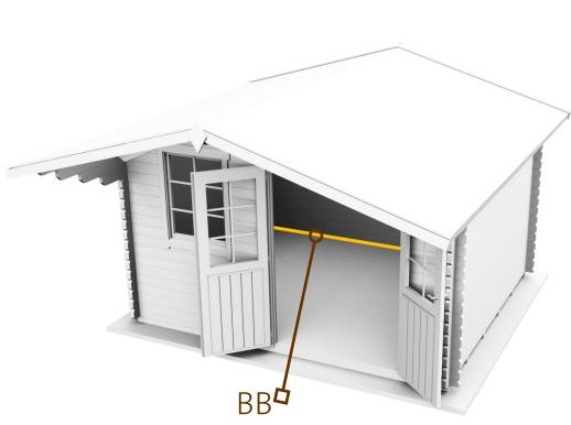
WINDBOARD CONNECTS BOTTOM LOG WITH THE TOP LOG. SAW THE WINDBOARD INTO THE RIGHT LENGTH. FOR THE TOP BOLT, DRILL 8MM HOLE THROUGH THE WINDBOARD.
