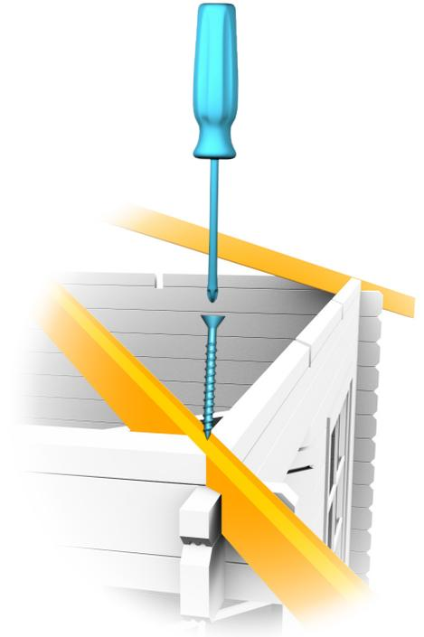
INSTALL THE ROOF PURLINS (RFB) AND ATTACH THEM WITH SCREWS.
