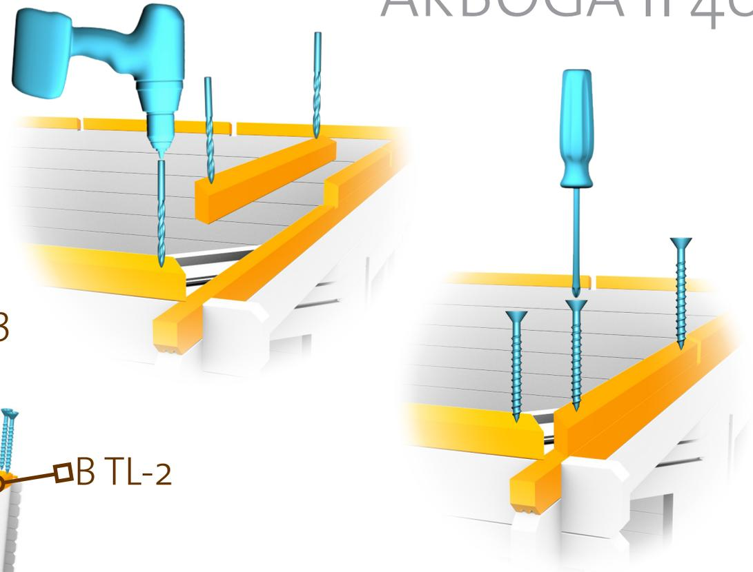
CONNECT THE ROOF PURLINS (RFR) WITH RD BEFORE INSTALLING THEM ON TOP OF THE CORNERS.
