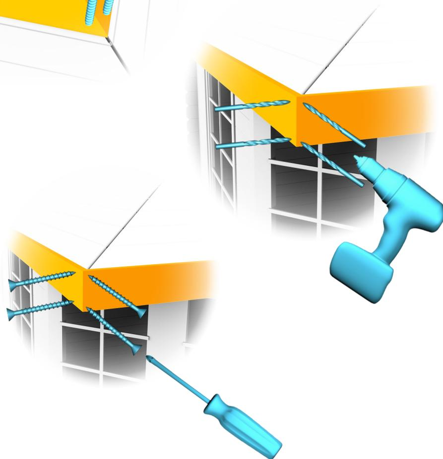
SCREW THE **FLOORBOARDS** INTO FOUNDATION, SAW THE LAST **BOARD** TO MAKE IT FIT.
