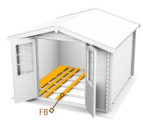
SAW THE BASEBOARDS AND ATTACH WITH NAILS AT EVERY 0,5 METERS.
