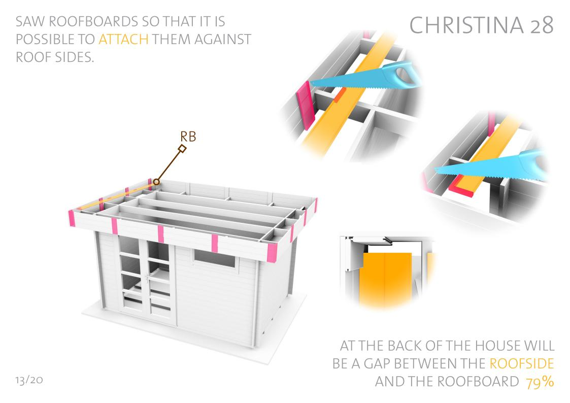
PLACE THE FIRST ROOFBOARD FLUSH WITH CHRISTINA 28 THE END OF THE PURLINS AND ATTACH WITH 8 SCREWS, 4 INTO EACH NEXT. RB
