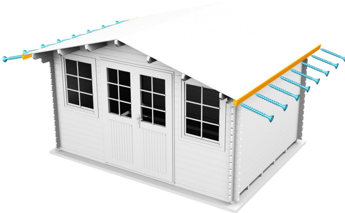
EAVES EDGES GO ON TOP OF THE ROOFING\*.
