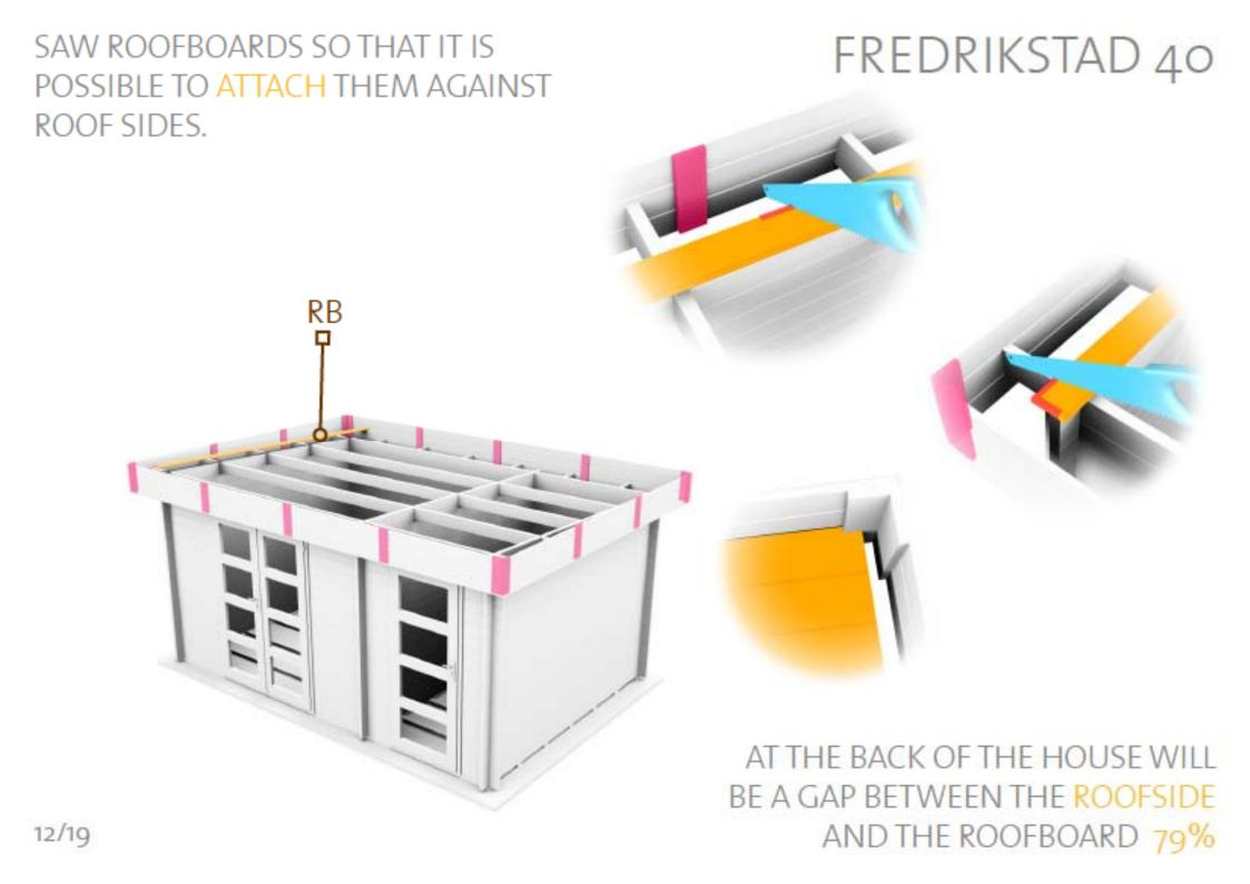
PLACE THE FIRST ROOFBOARD FLUSH WITH THE END OF THE PURLINS AND ATTACH
