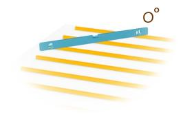
MAKE SURE THAT THE FOUNDATION IS INSTALLED ON A LEVEL SURFACE. CHECKING ALL DIRECTIONS, INCLUDING CORNER TO CORNER. 3%
