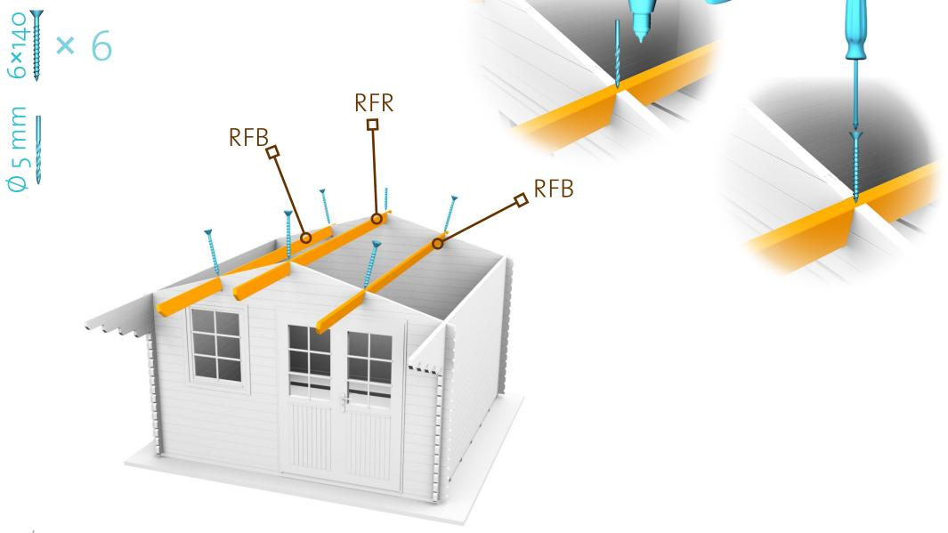
PLACE THE FIRST ROOFBOARD FLUSH WITH THE END OF THE PURLINS AND ATTACH WITH 6 SCREWS, 3 INTO EACH NEXT, SAW THE LAST BOARD TO MAKE IT FIT.
