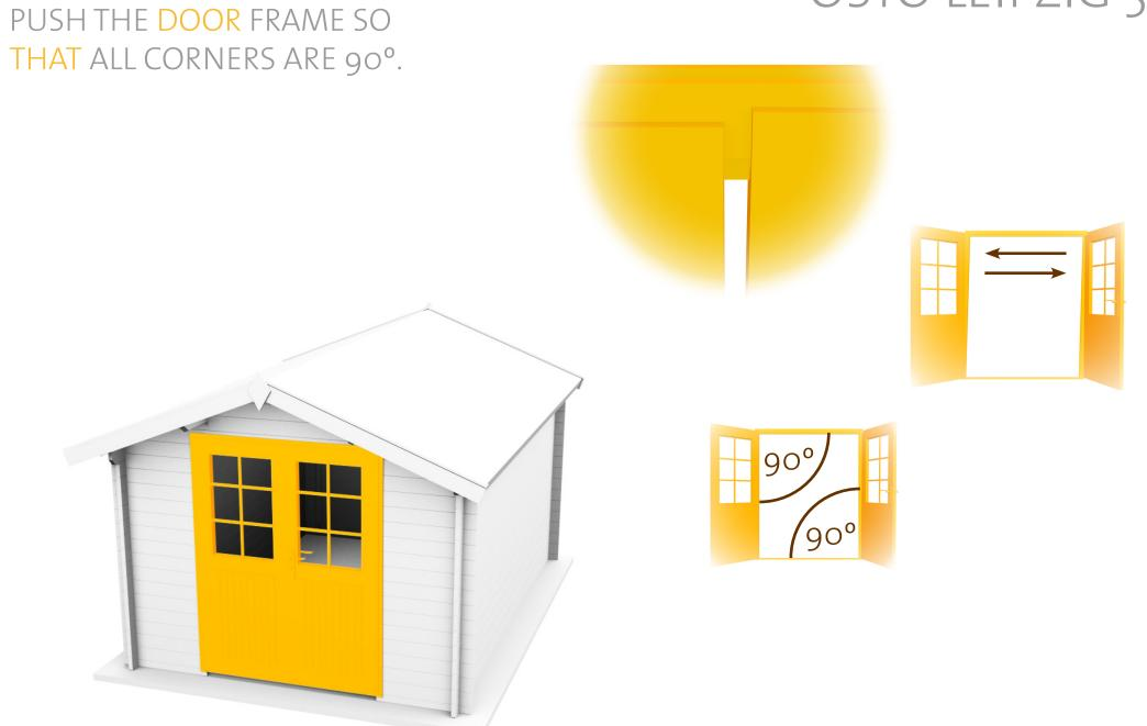
IF DOORS ARE IN DIFFERENT HEIGHTS OR THERE IS A GAP BETWEEN THEM, ADJUST 3 SCREWS ON DOOR HINGES.
