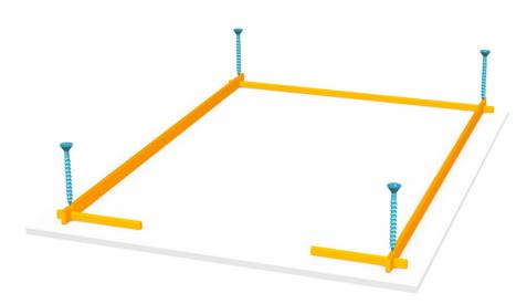
ATTACH THE FIRST ROW OF WALL LOGS INTO THE BOTTOM LOGS WITH SCREWS.
