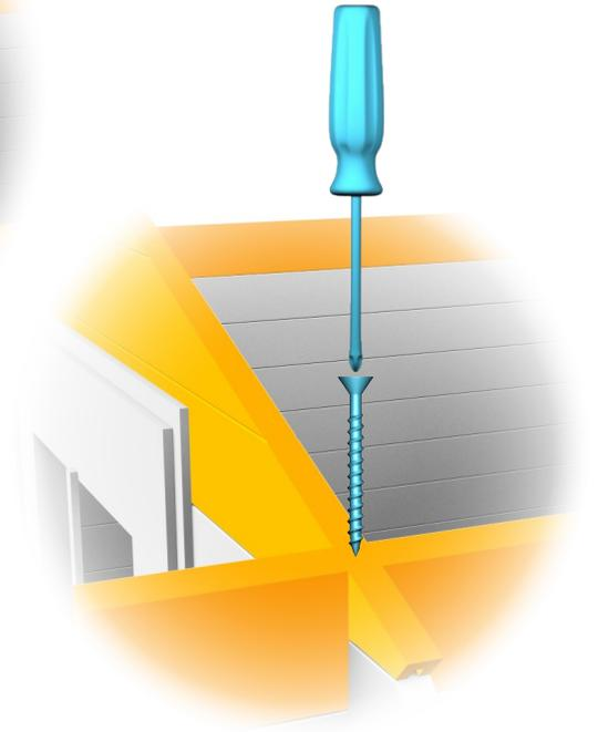
INSTALL THE **ROOF** PURLINS AND **ATTACH** THEM WITH SCREWS.
