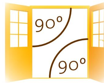
IF **DOORS** ARE IN DIFFERENT HEIGHTS OR THERE IS A GAP **BETWEEN** THEM, **ADJUST** 3 SCREWS ON DOOR HINGES.
