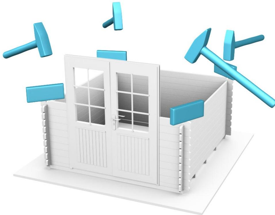
INSTALL THE GABLES WITH LONG SCREWS TO THE WALL LOGS ON THE FRONT AND REAR WALLS.
