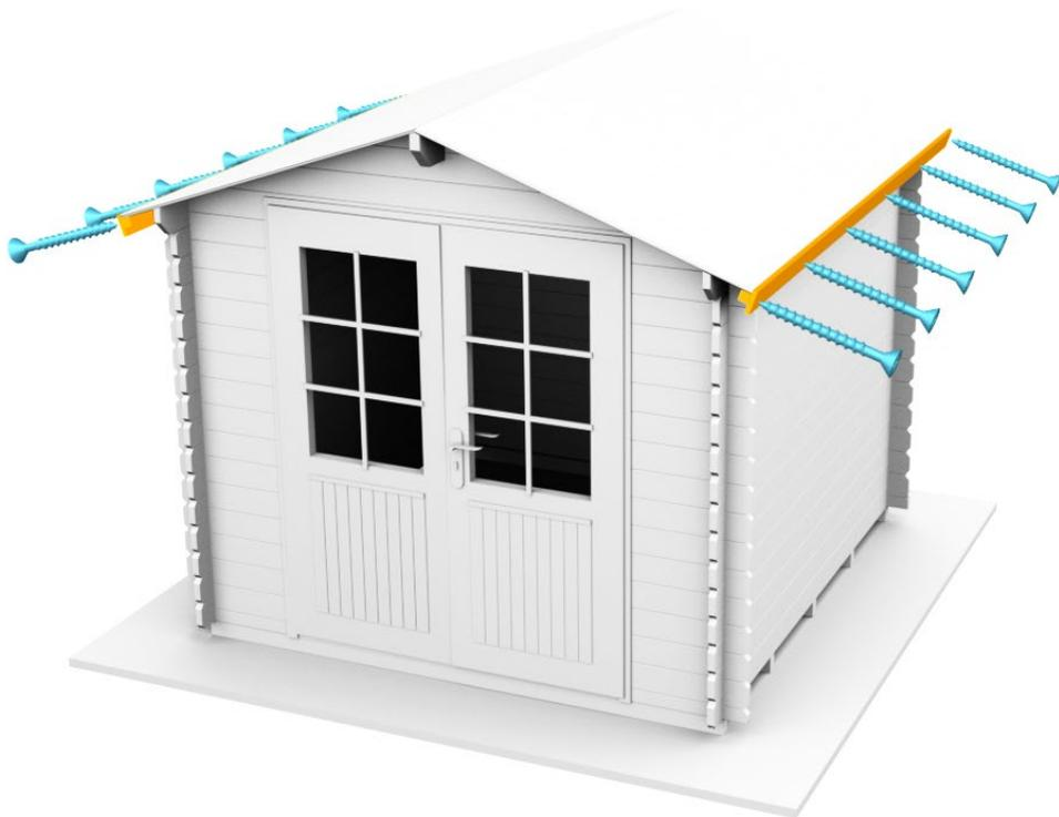
EAVES EDGES GO ON TOP OF THE ROOFING\*.
