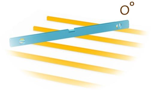
MAKE SURE THAT THE FOUNDATION IS INSTALLED ON A LEVEL SURFACE. CHECKING ALL DIRECTIONS, INCLUDING CORNER TO CORNER. 3%
