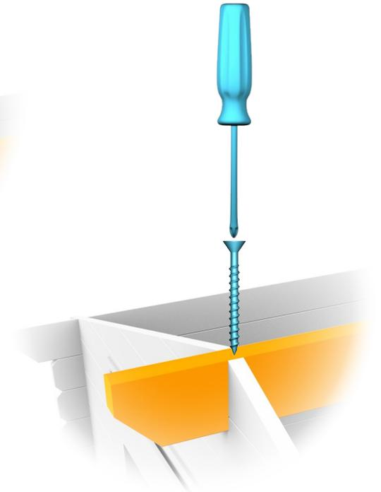
PLACE THE FIRST **ROOFBOARD** FLUSH WITH THE END OF THE **PURLINS** AND ATTACH WITH 6 SCREWS, 3 INTO **EACH** NEXT, SAW THE LAST **BOARD** TO MAKE IT FIT.
